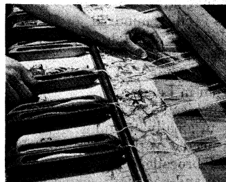
BY COURTESY OF THE SCALAMANDRE MUSEUM OF TEXTILES FIG. 3.—ITALIAN DESIGN LINEN DAMASK (FIG. 2) BEING BROCADED ON 50-IN. LOOM
